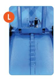
The lift has been specifically designed for the purpose of lifting electric vehicle battery during maintenance. It can also be used for engine or transmission work. All mechanical frames, including platforms, base frames, and arms, have been constructed using steel plates to ensure a robust and sturdy frame while minimizing overall weight. The lift comprises two tables, scissor arms, a base frame and a mobile jack.
