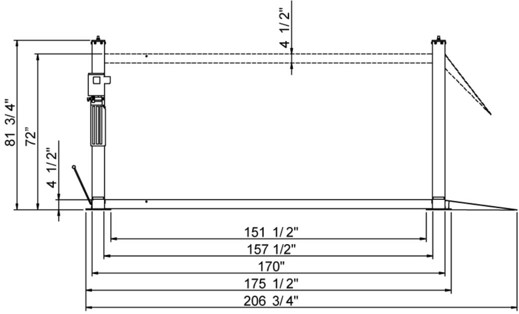
YOU WILL NEED A MIN. OF 6' CLEARANCE IN FRONT TO INSTALL HANDLE ROD
