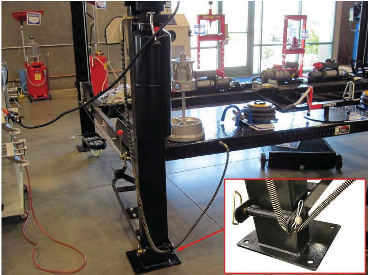
**Do not allow the hydraulic hose to get caught on the caster support rod. When you raise the lift the hydraulic line may be pulled from the power unit or the cylinder resulting in a HUGE oil spill. This is not covered by warranty Please pay attention.**
