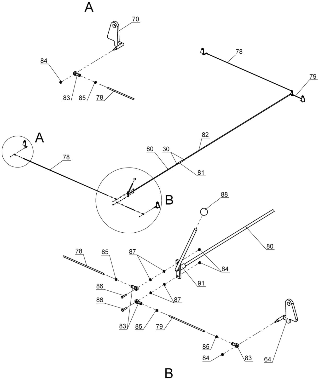
**SAFETY LATCH & LINKAGE COMPONENTS – FIGURE # 5**
