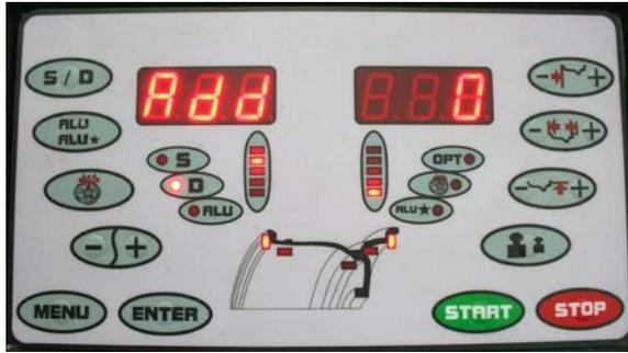
**STEP 9:** When the cycle is finished and the tire stops, the display will read “100 Add” (3.5 ounce). Rotate the wheel until all the inside weight indicators are fully lighted. Apply the 100 gram (3.5 ounce) calibration on the inside edge of the wheel at the 12 o’ clock position. Lower the hood and spin the wheel.
